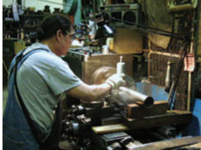
Quality Float Works employee Ramiro Bocanegra performs a trimming process using a lathe.
